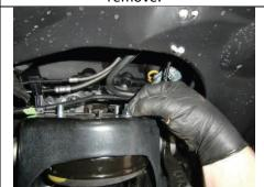
Use **SILVER Flange Nuts** to re-attach top of strut to vehicle.
