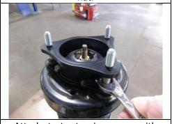
Attach strut extension spacer with **GOLD Flange Nuts**, tighten.
