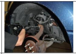
Loosen upper ball joint nut, but do not remove.
