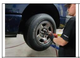
Lift vehicle securely and remove wheels/tires.
