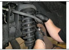
Pull down and remove upper ball joint nut.
