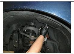
Loosen upper strut mount nuts.
