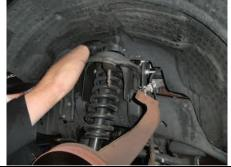
Remove top strut mount nuts and remove assembly.
