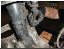
Reconnect lower sway bar end links and torque to spec.
