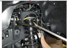
Use jack and pry bar to reattach upper ball joint to spindle.
