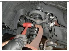
Carefully strike spindle as shown to separate ball joint.
