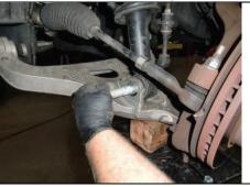
Reconnect lower strut mount and torque to spec.
