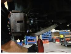
Remove lower sway bar end link hardware.
