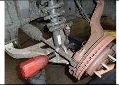
Loosen lower strut bolt/nut and remove.
