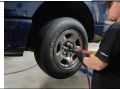
Lift vehicle securely and remove wheels/tires.
