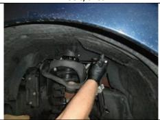
Loosen upper strut mount nuts.
