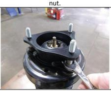
Attach strut extension spacer with **GOLD Flange Nuts** tighten.
