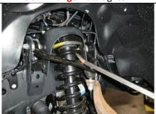
Use jack and pry bar to reattach upper ball joint to spindle.
