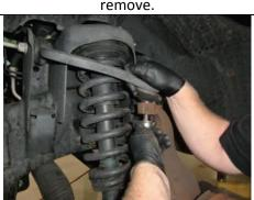
Pull down and remove upper ball joint
