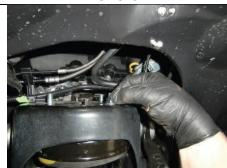
Use SILVER Flange Nuts to re-attach top of strut to vehicle.
