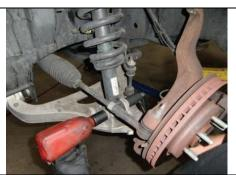
Loosen lower strut bolt/nut and remove.
