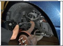
Loosen upper ball joint nut, but do not remove.
