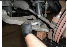
Reconnect lower strut mount and torque to spec.
