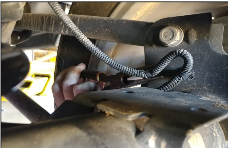
Remove the two ABS clips from the axle.
