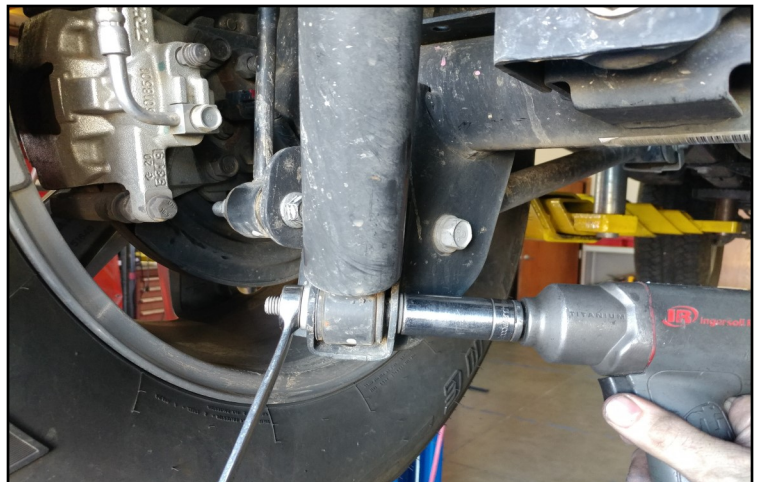
Remove the shock from the axle.
