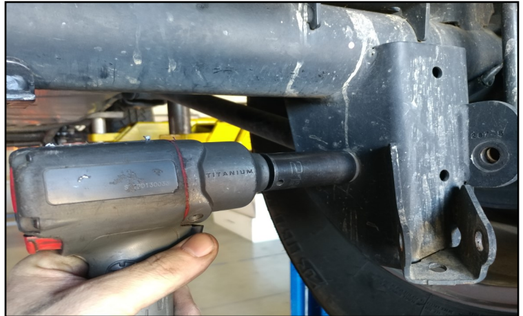
Loosen the control arms at the axle and frame.
