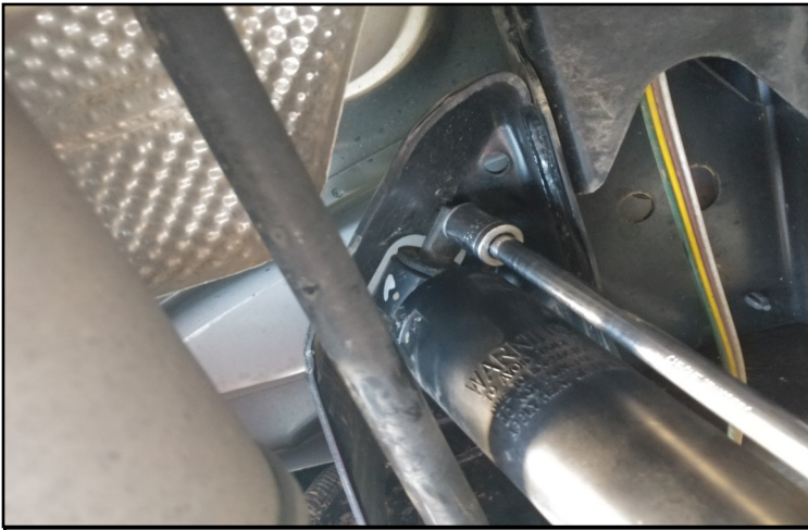
Remove the shock from the frame.
