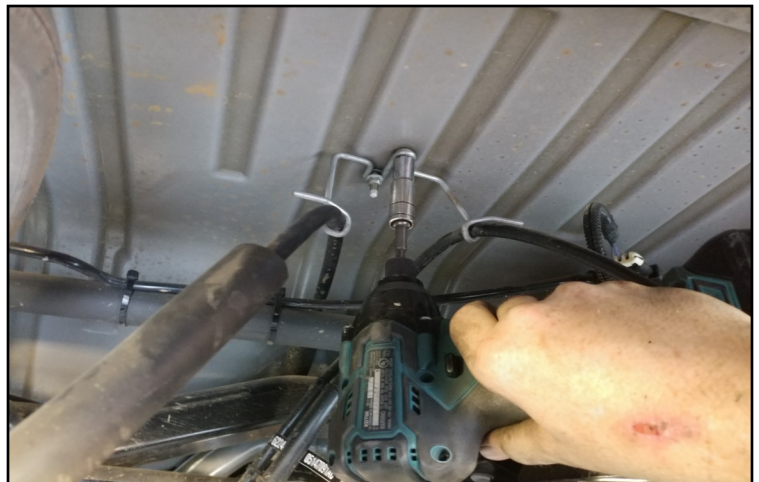
Remove the parking brake cable from the body.
