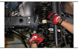
Carefully lower front axle enough to remove front spring
