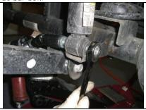
Disconnect and remove front lower shock hardware.
