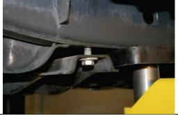
Loosen (2) front transfer case skid plate bolts.
