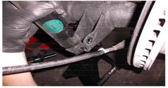
With the axle supported, unbolt the shocks from the axle.
