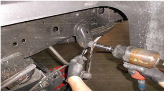
Unbolt the sway bar end links.
