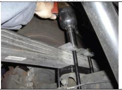
Raise axle, install new u-bolts and hardware, tighten.
