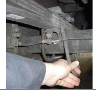
Remove u-bolts and carefully lower axle.
