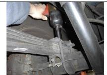
Work on one side of vehicle at a time, remove rear u-bolts.
