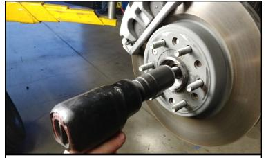
Remove the axle nut from the hub.
