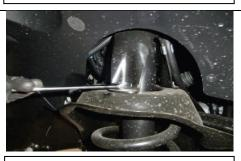
Loosen all (3) upper shock tower mounting nuts. Leave on.
