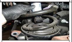
Slowly lower axle in order to remove shock and coil spring.
