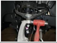
8. Using a pry bar, release tension, remove upper ball joint nut.
