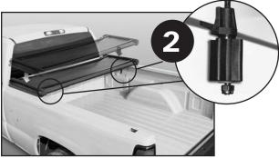
2. Secure cab clamp hooks under the metal bed rail.
