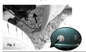
Using an easy removal tool, remove the push pins that holds the plastic protector (See Fig. 2)
