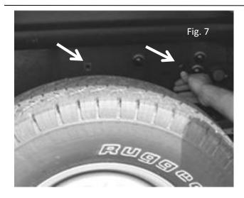
**8. For Trucks 2005 - 2008:** Insert one of the Medium size Push Pins into the pre-drilled holes attaching the liner to the truck frame (See fig. 7)
