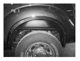
5. Insert the bottom sides and the upper section of the plastic liner behind the flange around the wheel well house edge. (See fig. 4)
