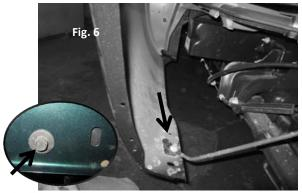
**8.** Insert one of the Medium size Push Pins into the pre-drilled hole attaching the liner to the truck frame (See fig. 7)
