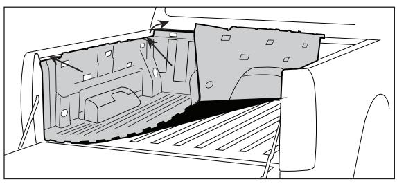
1. Insert the bedliner driver's side wall under the truck bed rail and partly over the bulkhead or front top of bed.
