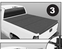
**3**. Unfold the cover all the way open to align cover on the truck bed rails before clamping.
