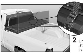
**2**. Undo both tie-down straps so cover can be unfolded.
