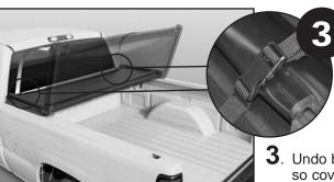
3. Undo both clips so cover can be unfolded.
