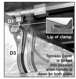
**2&7**. To clamp cover down, put lip of clamp under side bed rail and push handle down. (See D1, D2, D3)
