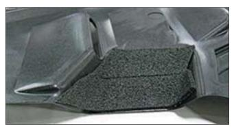
3. Install the LH coil cover (1318-6P067) in place over the LH side of the engine. Line up the bolt holes on the cover with the holes on the heater brackets. Route the lines coming out of the engine cover through the recess with the foam strip.
