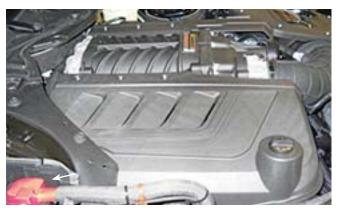
Install three (3) 18-8 button-head socket capscrews (92095A240) on the cover and torque to 7 Nm.
