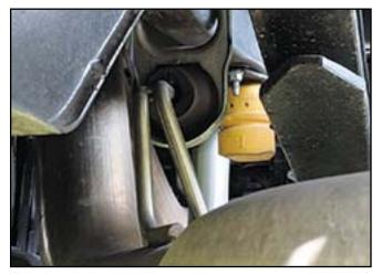
3. Push the front isolators onto the ROUSH system as shown and align to the factory studs.
