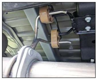
Install the three (3) 15 mm bolts removed in step 2 of the Disassembly section and torque to 55 Nm (41 ft lb).
