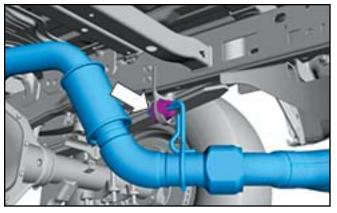
5. Remove the factory exhaust gasket.
