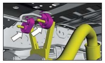
4. Slide the tailpipe assembly towards the rear of the vehicle, out of the isolator, and remove the assembly from the vehicle.
