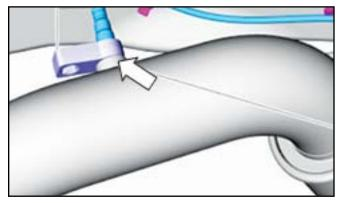
Remove the three (3) bolts from the flange securing the over axle pipe to the DPF flange (15 mm).
