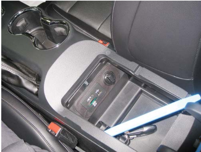
28. Release the clips for the shifter trim bezel and remove the top section of the center console from the vehicle.
