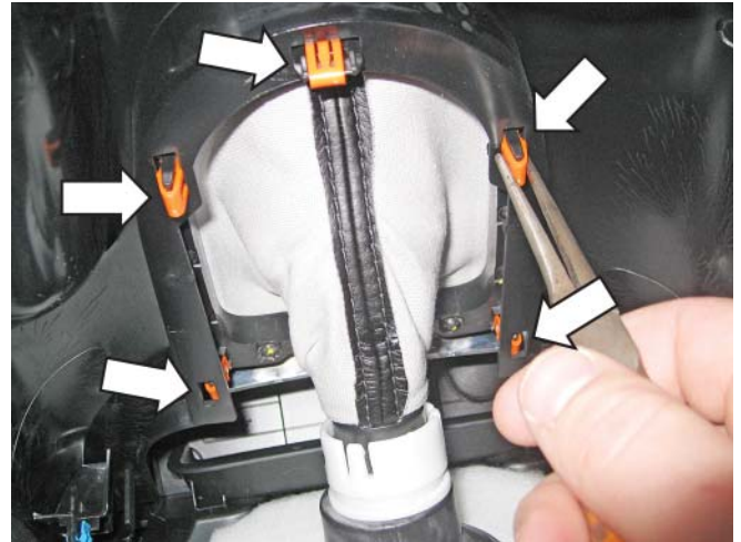
28. Release the clips for the shifter trim bezel and remove the top section of the center console from the vehicle.
