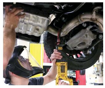
3. With the exhaust pipe cut, slide the hanger out of the rubber mount and remove the muffler/tip assembly from the vehicle.
