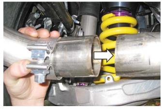
4. Slide the band clamp (94-0053/94-0052) over the joint in step 3 and torque the 15 mm bolt to 30 Nm.
