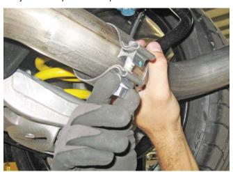
5. Place the band clamp (10-0338) over the exhaust tip and slide the tip over the muffler. Once the tip is in position, torque the band clamp to 30 Nm (V8 shown).
