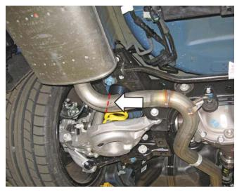
Cut the LH and RH exhaust pipes at the locations marked in step 1 using a reciprocating saw with a metal blade.
