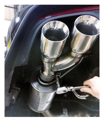
Check the exhaust system for correct clearance under the vehicle and also for tip alignment as shown below. If alignment is off, loosen the required band clamp, adjust, and re-torque the band clamp (V8 shown, I4 single tip).
