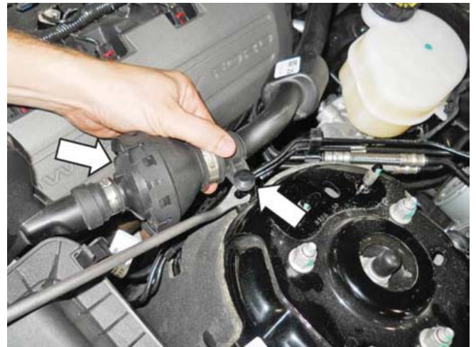
15. Remove the steel bushing followed by the two (2) rubber grommet from the stock air box tray. Retain these for use during installation.
