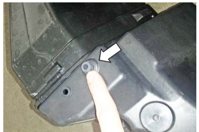
16. Remove the rubber isolator from the bottom of the stock air box tray and retain for use during installation.
