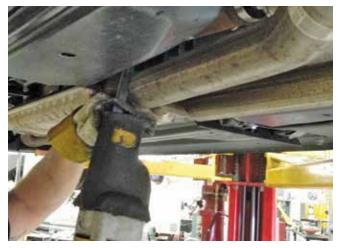
3. Loosen both of the OEM sleeve clamps in front of the resonator. These clamps are to remain on the vehicle.
