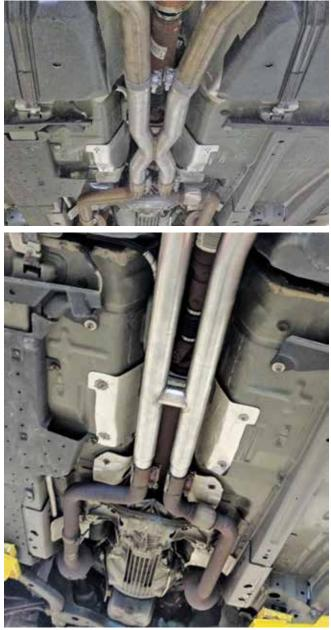
Before starting the vehicle, make sure to check all wires, hoses, brake lines, body parts, tires, and any other components for safe clearance from the exhaust system.
