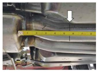
2. Cut the LH and RH exhaust pipes at the locations marked in step 1 using a suitable cutting tool.
