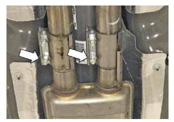
4. Push the rear exhaust pipes out of the way as needed and remove the resonator. This concludes the removal process for the OEM resonator.
