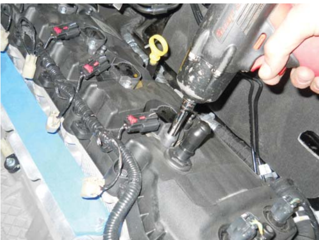
12. Remove the fasteners holding the ignition coils in place.
