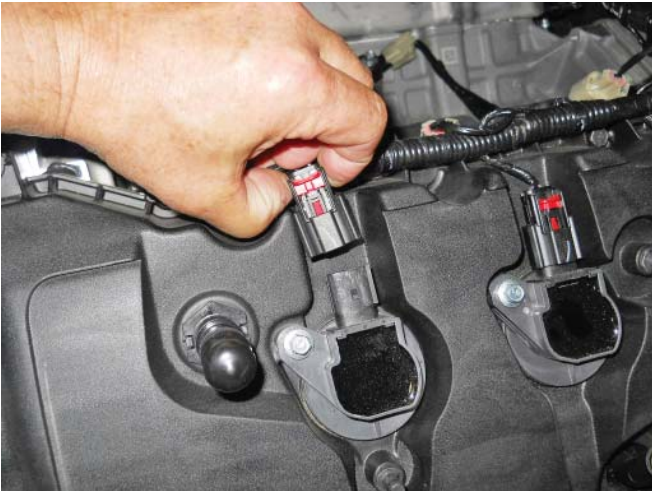
12. Remove the fasteners holding the ignition coils in place.
