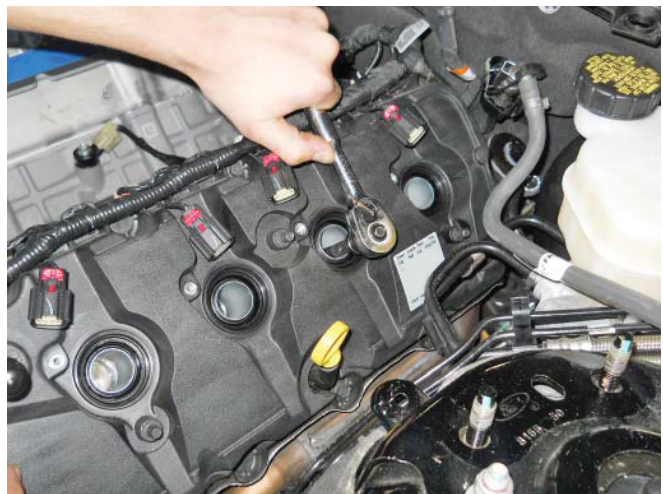
15. Unpack the eight (8) provided spark plugs (M-12405-M50), YOU MUST RE-GAP PLUGS TO 0.9 mm (.035") and verify that the plugs are not damaged.
