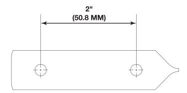
**Note:** Print this page at 100% scale and verify that the drill template has printed properly by measuring it after it is printed.
