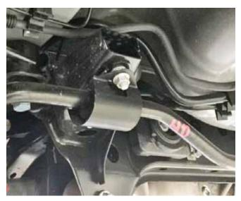
Locate the template onto the rear chassis sub frame as shown in the pictures below and mark the drill holes with a center punch. Use the same template to mark the holes on both the RH and LH sides of the vehicle.
