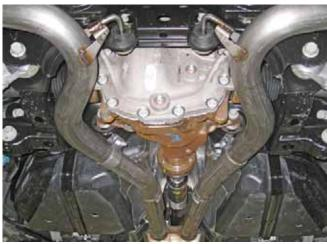
Slide each exhaust tip (P/N: 1315-AVTIP) onto the muffler outlets with the exhaust tip clamps (P/N: 10-0338). Align the tips to the rear valance. Torque the exhaust tip clamps to 35 lb-ft (47 Nm).
