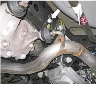
Unhook each exhaust hanger from the sub frame and remove each muffler assembly by sliding the inlets down and forward to extract the rear exhaust hangers from their mounts.
