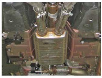
8. Install each side of the ROUSH exhaust system by inserting the rear exhaust hangers first and then sliding each side forward to fully seat the inlets with the forward section of the stock exhaust. Be sure to connect the rubber isolators to the hangers that were installed in step 7 and also reinstall the two (2) IRS sub frame exhaust hangers with the two (2) 13 mm bolts that were removed in step 2 and torque to 18 lb-ft (25 Nm). Torque the exhaust pipe clamps to 35 lb-ft (47 Nm).
