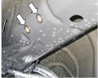
5. Install the two (2) supplied exhaust hangers (P/N: 1315-5A261 and 1315-5G298) and four (4) bolts (P/N: W500224) as shown below. Torque to 18 lb-ft (25 Nm).
