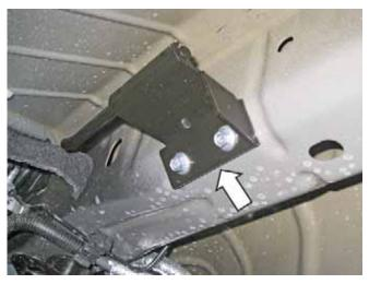
Remove the two (2) IRS sub frame mounted exhaust hangers from the stock exhaust system and slide them onto each side of the ROUSH exhaust.
