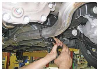
2. Remove the two (2) 13 mm bolts that retain the exhaust hangers on the IRS sub frame.
