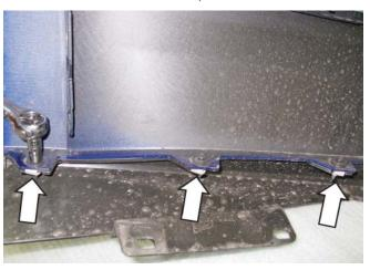
21. Remove the lower bumper cover trim piece by releasing the twenty-two (22) retaining tabs.
