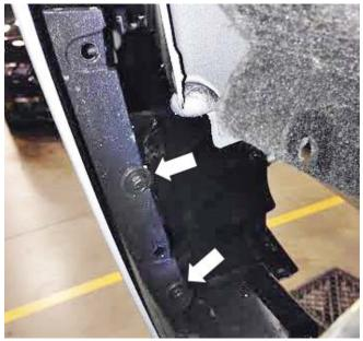
5. Remove two (2) push-in retainers under each side of the rear bumper behind the rear tires.
