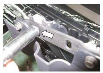
39. Install one (1) bracket (P/N: 1315-17F950), one (1) J-clip (P/N: N623332-S439), two (2) 7m screws (P/N: 98093A316) and one (1) 10mm screw (P/N: 98093A440) onto each side of the lower rear valance in order to secure it to the bumper cover reinforcement piece.
