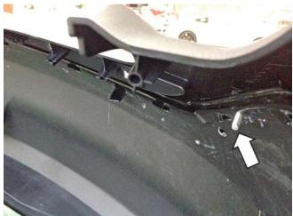
31. Loosely install eleven (11) screws (P/N: 99397A767) into the top row of holes. Loosely install two (2) screws (P/N: 90925A245) with two (2) washers (P/N: 1133153) into the top outer corners while being sure to properly align each hole with the plastic bosses on the valance.
