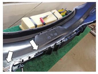
Apply 3M Ad-Pro<sup>®</sup> (P/N: 021200-27571) onto the rear edges of the side valance pieces (P/N: 1315-17F955 & 1315-17F956) and then install the 2-sided tape (P/N: TAPE-015-12.5x68).
