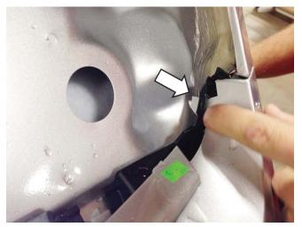
10. Hold the center of the bumper cover and partially remove it in order to gain access to remove the wiring harness connector under the RH tail lamp. With the connector removed, remove the bumper cover and place it on a protective surface.
