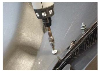
32. Remove the backing off the 2-sided tape, apply blue Loctite<sup>®</sup> to the threads on the studs that were installed in step 24 and then torque all of the fasteners that were installed in steps 24-26 to 0.7-0.8 Nm.
