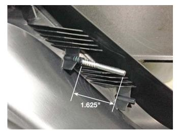
30. Place the rear valance on the bumper cover by first aligning the two outer studs with the lower outer holes drilled in step 21. Loosely install one washer (P/N: 1133153) and one nut (P/N: 90480A011) onto each stud and then lay the back of the rear bumper cover down onto a protective surface
