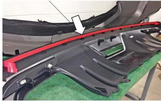
29. Peel a small portion of the backing off the doublesided tape on each end in order to create "flags" that will allow for complete removal once the valance is secured into position. Install two (2) studs (P/N: 90207A253) into the outer middle bosses on each side of the rear valance and to the correct depth as shown.
