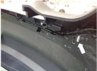
Loosely install eleven (11) screws (P/N: 99397A767) into the top row of holes. Loosely install two (2) screws (P/N: 90925A245) with two (2) washers (P/N: 1133153) into the top outer corners while being sure to properly align each hole with the plastic bosses on the valance.
