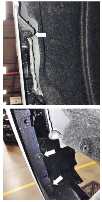
5. Remove two (2) push-in retainers under each side of the rear bumper behind the rear tires.
