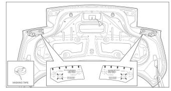
7. Create four (4) access holes in the trunk's inner sheet metal by center punching four (4) hole locations, two (2) per side. Drill each center punched location with a 1/8" drill bit. Enlarge each 1/8" hole with a 1.0" hole saw.
