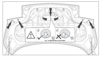
14. If the fasteners and holes are not aligned, remove the rear spoiler and use a round file to adjust the holes in the trunk lid outer sheet metal accordingly.
