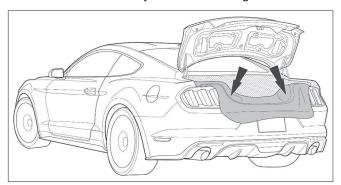
5. Carefully cut out the LH and RH inner drill templates from the larger template sheet (1315-SPLRTMPL).
