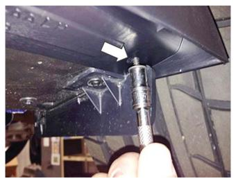
6. Install the front self-tapping mounting screw with a 7 mm socket. Torque to 1.0 Nm.
