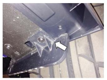
3. Align the winglet parallel with the rocker panel edge and then mark each mounting hole.
