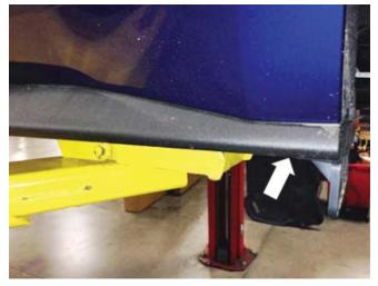
2. Spread the factory rear rocker trim piece apart from the rocker panel and insert the rocker winglet into the opening until it is fully seated.
