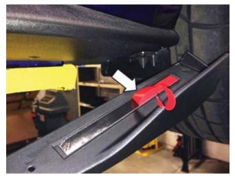
5. Reinstall the winglet and line it up with the previously marked holes. Install the rear self-tapping mounting screw with a 7 mm socket. Torque to 1.0 Nm.
