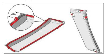
Install the side scoop onto the body side using the directions on the template. Do not allow the exposed double-sided tape to adhere to the sheet metal until the side scoop is properly aligned, then press down.
