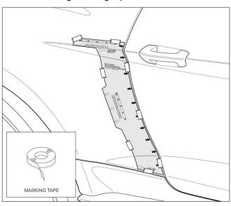
5. Peel back 2.0" (50.0 mm) of each tape liner and secure to the A-side of the side scoop with masking tape.
