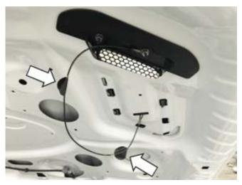
Remove two (2) 9 mm nuts, release the retaining clips and remove each factory heat extractor.
