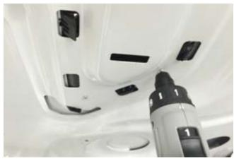
10. Reinstall the factory black plastic brackets with the two (2) nuts that were removed in step 3. Torque them to 1.4 Nm.
