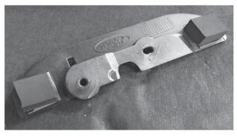
8. Remove the two (2) studs from the factory heat extractors and install them on the ROUSH Heat Extractors.
