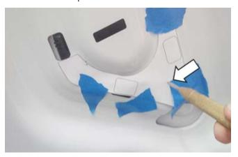
6. Drill each hole with a 1/8" bit. After the holes are drilled, apply commercially available clear coat (Motorcraft Part Number: PM-19500-6000) to the exposed metal so that it does not corrode.
