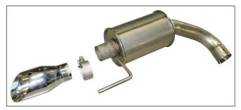
Check the exhaust system for correct clearance under the vehicle and also for tip alignment as shown below. If alignment is off, loosen the required band clamp, adjust, and re-torque the band clamp.
