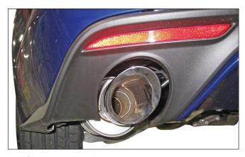
Once the desired position and alignment have been achieved, make sure all band clamps are torqued to 30 Nm.
