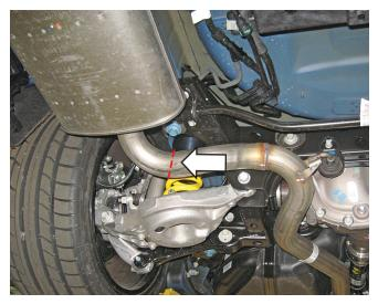
2. Cut the LH and RH exhaust pipes at the locations marked in step 1 using a reciprocating saw with a metal blade.
