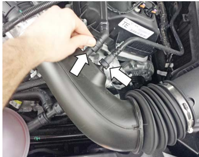
9. Remove the clamp on throttle body end of the clean air tube and remove the air tube.
