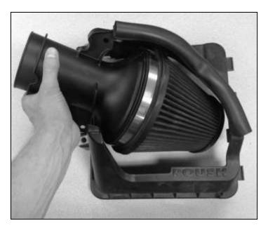
9. Install the EPDM close out seal (1111-9645) around the MAP Tube and clip into the edges of the upper air box tray.
