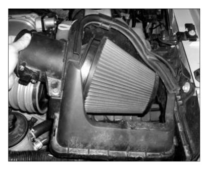
13. Connect the clean air tube to the new ROUSH air box lid assembly. Secure the clamps for the air box lid and tighten the clamp on the clean air tube to the MAP Tube.
