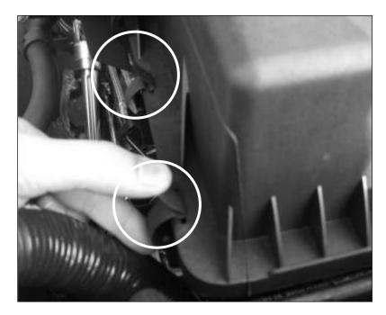
5. Transfer the MAP sensor from the factory air box lid to the new ROUSH MAP tube (1113-12B579) and fasten it with the supplied bolt (M19-013-0018). Torque the bolt to 1.8 - 2.2 Nm.
