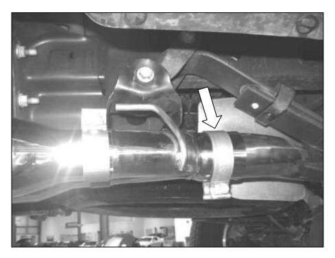
13. Insert the Y-pipe hanger into the hanger bracket. It is important to note the orientation of the bracket as it will hang underneath the suspension bracket.
