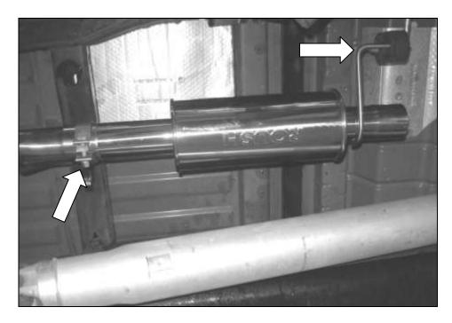
5. Position the intermediate pipe (1111-5246) into the catalyst adapter flange.
