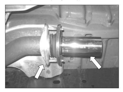
3. Position the new muffler outlet axle pipe (1111-5C262) into position and install the steel hanger brackets into the factory rubber hangers. Orient the pipe such that the flared end faces forward in vehicle.
