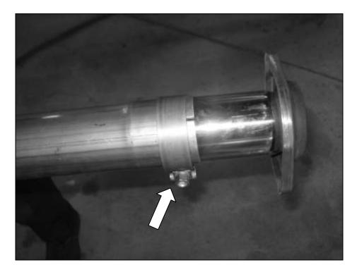
9. Insert one (1) 3" clamp (R12060012) over the end of the intermediate pipe and insert the intermediate pipe into the muffler. Position the clamp on the pipe joint and loosely secure.
