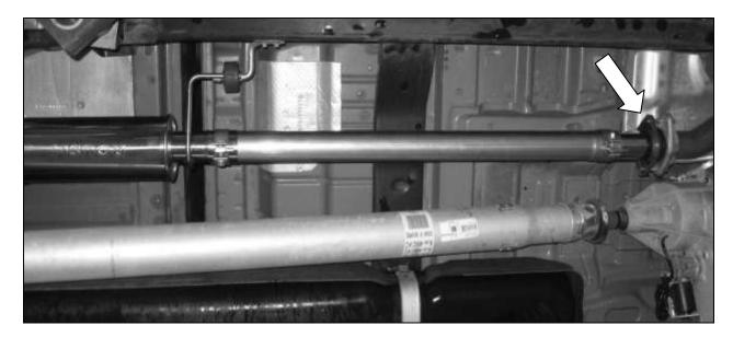
11. Install one (1) 2.5" clamp (R12060014) onto each of the exhaust tips and slide the tips onto the ends of the Y-pipe. Position the clamps on the pipe joints and loosely secure the clamps.
