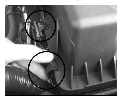
7. Transfer the MAF sensor and fasteners from the factory air box lid to the new ROUSH MAF tube (1111-12B579). Torque bolts to 1.8 - 2.2 Nm.
