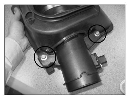
13. Orient the filter so it sits at a slight angle forward as shown.
