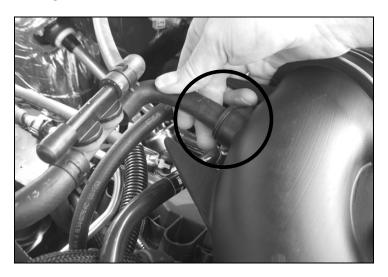
2. Disconnect the PCV line fitting from the clean air tube.
