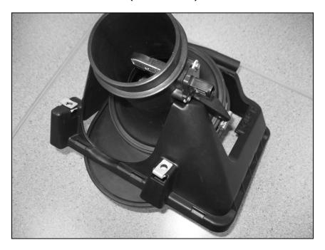
12. Install the EPDM close out seal (1111-9645) around the MAF Tube and clip into the edges of the upper air box tray.
