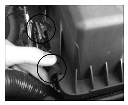
8. Transfer the MAF sensor and fasteners from the factory air box lid to the new ROUSH MAF tube (1111-12B579). Torque bolts to 1.8-2.2 Nm.
