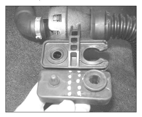
4. Place the rubber grommet onto the top surface of the tube mounting bracket. Re-install the steel insert from the bottom as shown.
