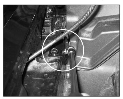
13. Raise the hood upward (to increase travel) and insert the opposite end of the strut onto the hood mounting brackets on either side.
