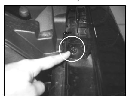
5. Install the left hand fender bracket (1312-LHFNDR), re-install the factory bolt and torque to 20 Nm.
