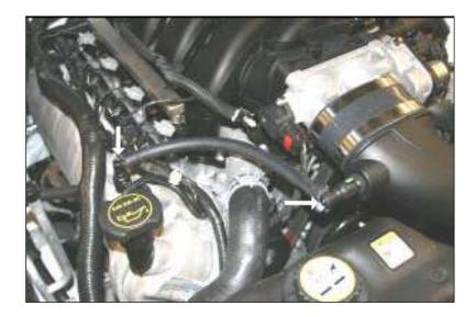
19. Install the new <u>Breather Hose</u> <u>Assembly</u> as shown.
