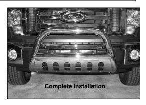
**NOTICE** Bull Bar may interfere with the performance of forward facing cameras and sensors, if equipped.
