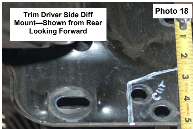
Trim Driver Side Diff Mount—Shown from Rear Looking Forward
