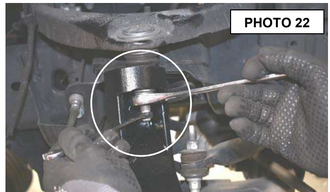
Tighten the upper ball joint using a 21mm & 10mm.
