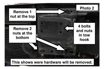
3. Remove the 4 bolts and nuts from the tow hook using a 18mm wrench and socket. See Photo 3 and 4.
