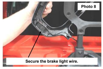
8. Make sure the wire is clear of the bottom mounting hole and install the back half onto the front half of the brake light mount, using the factory hardware. Tighten using a T25. **See Photos 9 & 10.**
