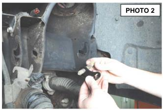
2. Using a 21mm socket and wrench remove the factory upper control arm bolts. Remove the factory cam plate as shown in **Photo 1.** Insert the new cam plate onto the bolt as shown in **Photo 2.**
