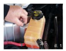
Remove the coolant reservoir cap. Using pliers, Squeeze the ears together on the hose clamp as shown in ill. 2. With the clamp squeezed open, use your other hand to remove the hose from the reservoir. Remove the clamp and set aside for reinstallation.
