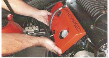
sure it is fully engaged. Without starting the car, we recommend you "key up" the car at this time. This will allow the fuel pump to start and you can visually check for leaks. If you have no leaks, turn the key off and continue with the installation.
