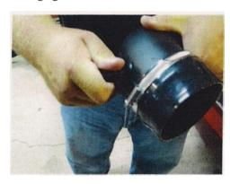
Step 6. Locate #21 Foam Seal. Install lower air box foam seal. Wipe area with supplied alcohol swab before installing seal. Install around the perimeter of air inlet hole on the car as shown in illustration.
