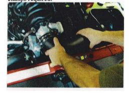
Step 12. Locate #6 air filter. Install Air filter. Align air filter inside the air box with the filter housing. Press filter until the seal is completely covering the filter housing. Using an 8mm socket, tighten hose clamp to secure the air filter in place. \*Note: Do not exceed 8 inch lbs. of torque.
