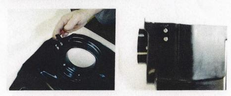
Step 9. Locate #14 Coolant Reservoir Bracket. Install the Coolant Reservoir Bracket. Using the supplied 10-32 SS machine screws, fasten the bracket to the back side of the Roto-Fab air box. \*Note: Install the head of the machine screws from the inside of the air box.
