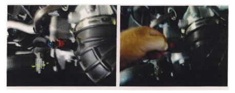
Step 3. Remove OEM air box. Using a 8mm socket, loosen hose clamp that holds the stock air tube to the throttle body. Next, use a 10mm socket to remove the air box bolt. Disconnect the breather hose, and remove the OEM air box assembly and air tube.
