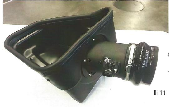
Locate the #9 4"- 4 1/4" step hose coupler and one of the smaller #10 hose clamps with 100-120MM stamped on it. Orient the clamp as shown. Fully engage the small end of the coupler onto the throttle body. Be sure the coupler is engaged on the bottom side of the throttle body. Tighten the clamp while positioned as shown with the 7mm head facing upwards. (see ill 12)
