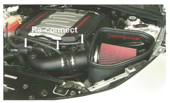
Congratulations, your installation is now complete! All clamps should be checked after a few drive cycles and periodically thereafter. Tighten as necessary. Your air filter will last for the life of your vehicle with periodic service. The service technique will depend on whether you have a dry or oil filter.
