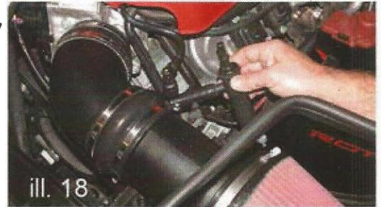
7) Re-connect the fitting to the top side of the breather by pushing it straight down until a "click" is heard.
