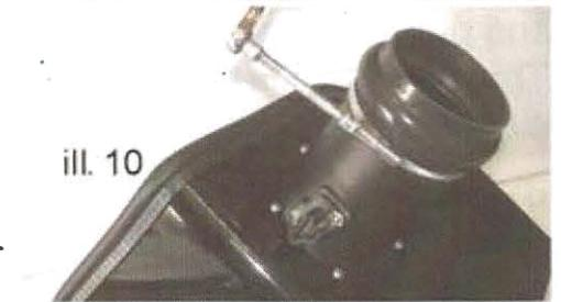
6) Locate the # 2 air filter with clamp. Engage the filter onto the large end of the MAF housing with the clamp oriented in the same manner as the clamp on the hump hose.
