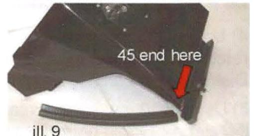
4) Locate the # 7 hood seal. Install it on the top edge of the air box. It is not necessary to fully seat it at this time.
