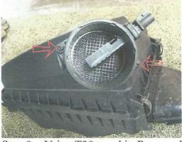
Step 9. Using T30 torx bit. Remove lower air box stud. See picture for details.
