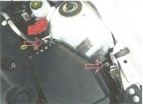
Step 5. Remove air box assembly. Using both hands, Pull firmly straight up to remove box. Note\* There is a grommet on the bottom side holding air box in place.
