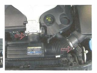
Step 2. Disconnect MAF sensor connector. Using your fingers, squeeze and pull firmly to disconnect the MAF sensor harness and remove MAF sensor.
