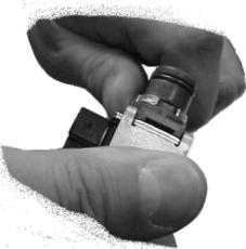
Install the new solenoids as shown, taking care to install the harness in the correct solenoids.
